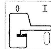
A spring presses the gear shift lever into a locking recess. In this position the band brake is slightly released and does not produce any braking action during the wind-up.
