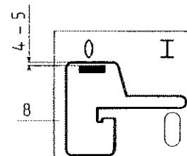
Turn the hex. nuts (6) on the threaded rod (7) apart until the spacing between the shifting gate (8) and the shut-off lever (9) is about 4 to 5 mm.
