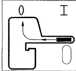
and slacken the PE-pipe by carefully pressing the shut-off lever downward.
