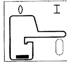
In this position the brake band must be slightly lifted off the brake disk. This prevents the brake band from sticking to the brake disk.
