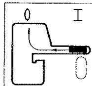
Slacken the PE-pipe by pushing down the gear shift lever carefully.
