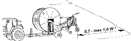
Drive the Rainstar machine into the field allowing for the sprinkler's distance of throw.
